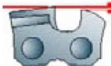
.025" (0.64mm) Depth-gauge Setting
